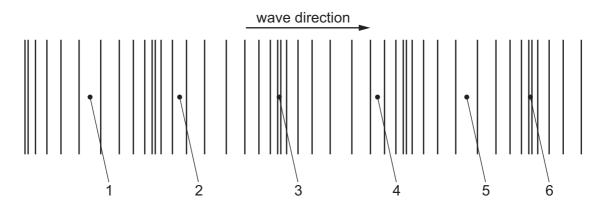
Which numbered points are at the centre of a compression and which numbered points are at the centre of a rarefaction?
