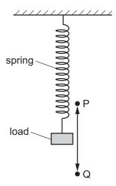
The load is pulled down and then released so that it oscillates between point P (highest point) and point Q (lowest point).
